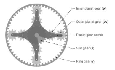
Structurally, the double-pinion planetary gear resembles a Ravigneaux gear without its second, large, sun gear. The inner planet gears mesh with the sun gear and the outer
