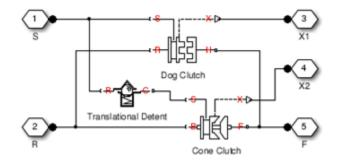
The model implements Dog Clutch, Translational Detent and a modified version of Cone Clutch blocks. Refer to each block reference page for more information on the corresponding block function. You can use a similar approach to model customized versions of the synchronizer. One example is the Gearbox (Detailed) subsystem in the model sdl\_manual\_transmission.
