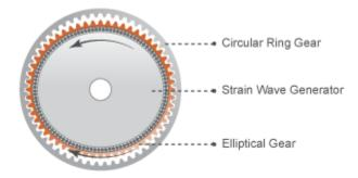
During normal operation, the base shaft drives the strain wave generator. The elliptical plug spins freely inside the elastic metal gear, propagating the strain wave about the gear rotation axis. This strain wave causes the elliptical gear teeth to progressively engage the internal teeth of the circular ring gear.
