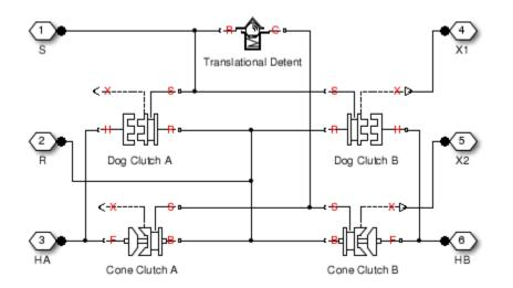
The model implements two Dog Clutch blocks, one Translational Detent, and two modified Dog Clutch blocks. Refer to each block reference page for more information on the corresponding block function.
