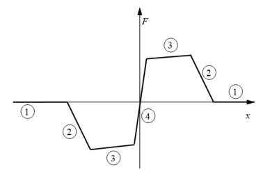
Because the ball is spherical and the notch is symmetric, the horizontal force versus displacement function is symmetric about the origin. (See "Peak Force and Notch Width" on page 1-338.)
