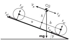
This figure and table define the vehicle motion model variables.
