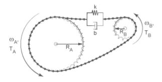
The chain tensile force is the net sum of spring and damper forces. The spring force is the product of the tensile strain and the spring stiffness constant. This force is zero whenever the tensile strain is smaller than the chain slack. The damper force is the product of the tensile strain rate and the damping coefficient. Mathematically,
