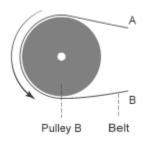
The block dialog box enables you to select the relative belt direction of motion. Depending on the chosen setting, the two belt ends can move in equal or opposite directions. The block model assumes noncompliance in the belt and no resistance to motion due to wrapping around the pulley.
