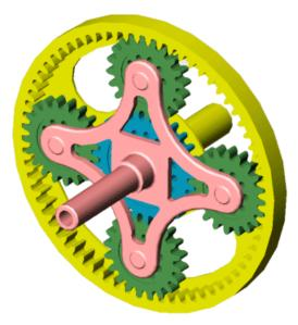
Depending on which shaft is driving, driven, or fixed, the planetary gear train can achieve a variety of speed reduction ratios. These ratios are a function of the sun and ring radii, and therefore of their tooth numbers. You specify the tooth numbers directly in the block dialog box.
